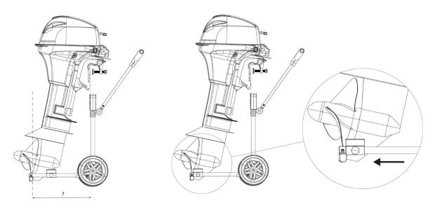
Now the trolley is set up for your engine. This does not need to be changed when you only use this specific engine on the trolley.
