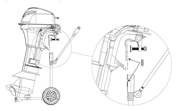
Step 4. Measure the horizontal distance between the bracket and the end of the engine tail.
